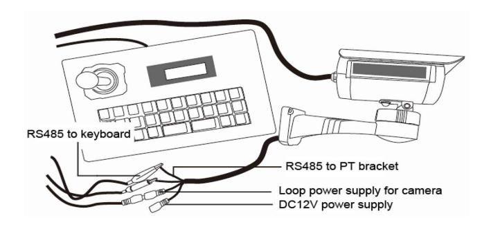
(2) Work with IP cameras, required the camera has RS485 port, support PELCO-D protocol.
